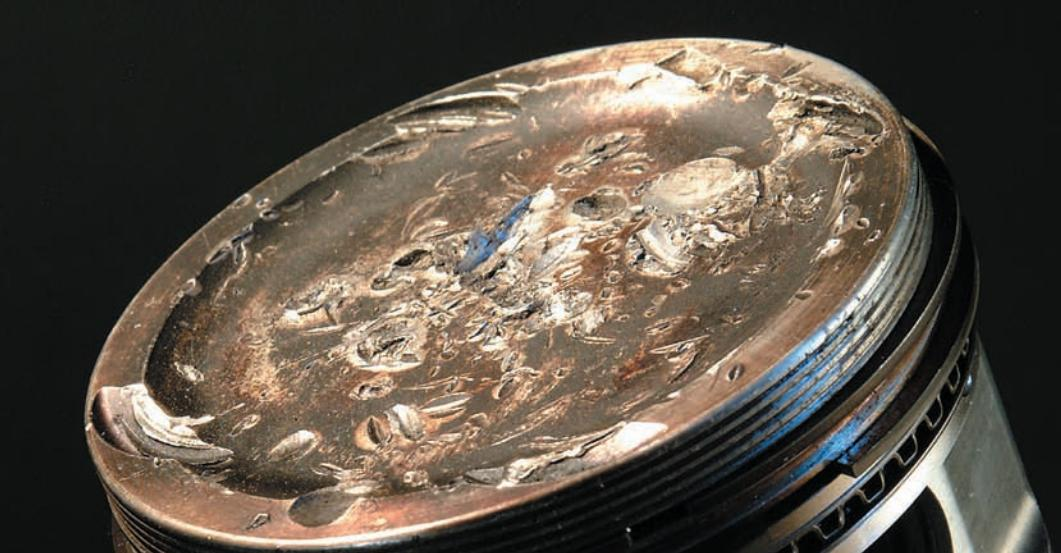
Cylinder head, valve train and piston damage due to lack of timing drive system maintenance.
